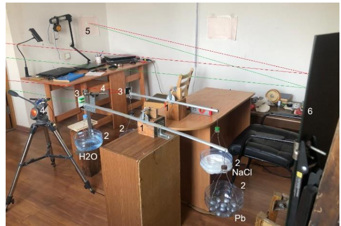
Figure 5. An experiment with two vertical pendulums. The photograph shows trajectories of two laser beams reflected by a system of mirrors and projected onto a common screen (5).
